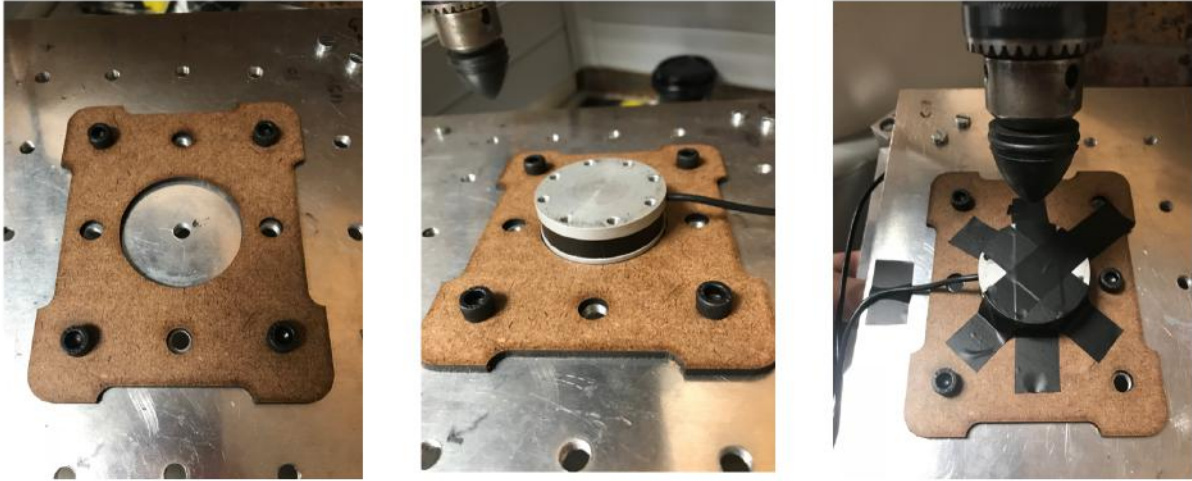
Figure 4.4: Images showing the OF sensor mounting brace used to prevent unwanted lateral translation during application of multi-axial forces. The right-most image shows the application of insulation tape used to prevent unwanted rotation of the OF sensor.
