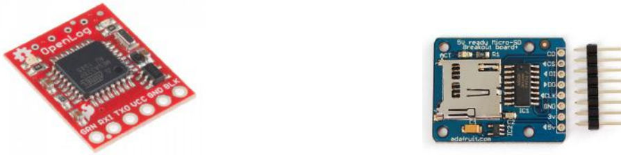
(a) Sparkfun OpenLog micro SD card breakout [59] (b) Adafruit micro SD card SPI breakout [58]
