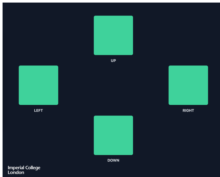
Figure 5.1: Screen capture of the user interface for displaying SSVEP stimuli. The blocks can be independently set to any flicker frequency of interest.
