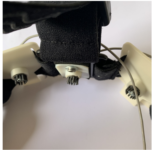
(b) Close-up view of the two active electrodes on either side of the reference electrode. Electrodes are housed in 3D-printed locator structures that allow for slight pitch and yaw deviations about the axis normal to the scalp.
